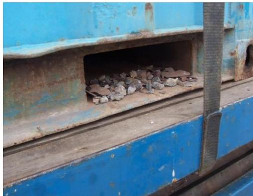
Figure 4 - debris- stones in forklift pocket
