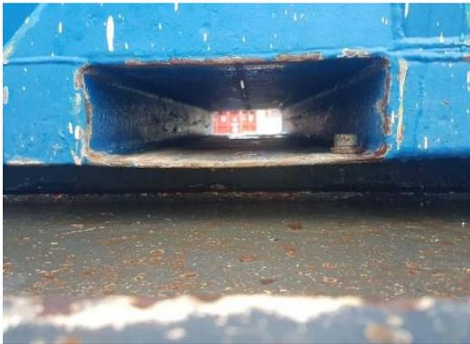
Figure 1 - nut in forklift pocket
