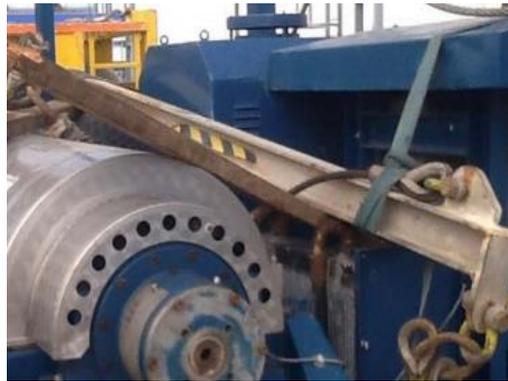
Figure 2 - Wooden beam not secured
