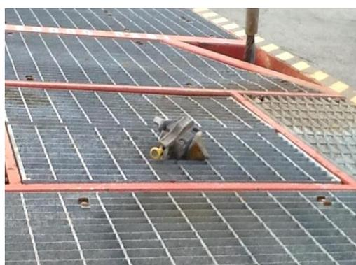
Figure 6 - Twist-lock on top of tank
